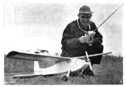
Mr. Blackie with one of his model planes. Powered by a  $2\frac{1}{2}$  c.c. glowplug motor it was made by him out of balsa, 3 ply wood and nylon fabric.
