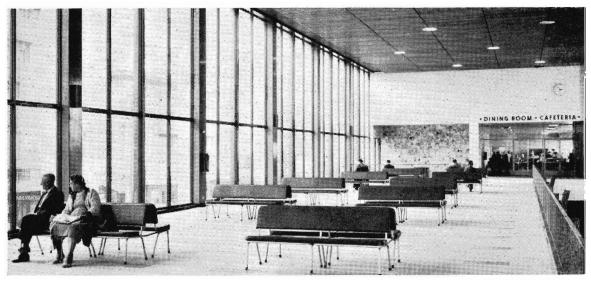
The Waiting Gallery, facing the street. A sound absorbing ceiling, and heavy plate glass in the window wall reduce traffic din. The glass is also tinted to subdue glare.
