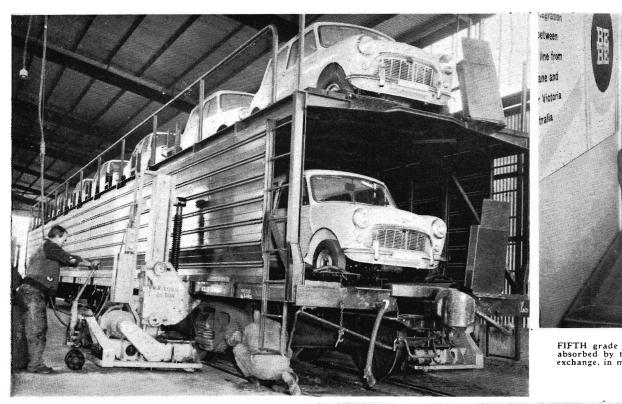
RAILING CARS: This two tier car-carrying BKX rail wagon was the first fully loaded New South Wales vehicle of its type to pass through the Bogie Exchange Centre at South Dynon. The motor cars were destined for Western Australia—a total journey of 2.692 miles. The N.S.W. Railways will. ultimately, have 38 modern car-carrying wagons available to handle the expanding motor car and body traffic that at one time was extensively handled by road.
