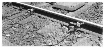
Micro switches mounted on rail
