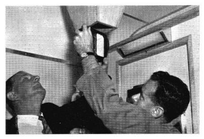
Using a velometer, Engineer H. Robinson (*left*) and Assistant Engineer W. Hoole check air flow. The pyramid shaped box is placed over the ceiling panel to measure the amount of air coming into the compartment from the air-conditioning unit. The velometer measures the velocity of the air.
