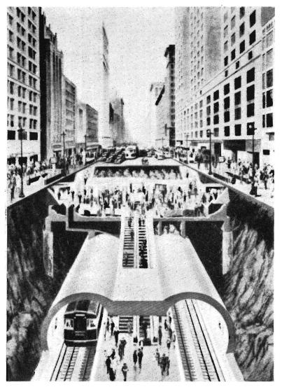
Cut-away drawing of Chicago's Underground. Four tunnels, carrying one track each, are proposed for Melbourne's City Underground.
