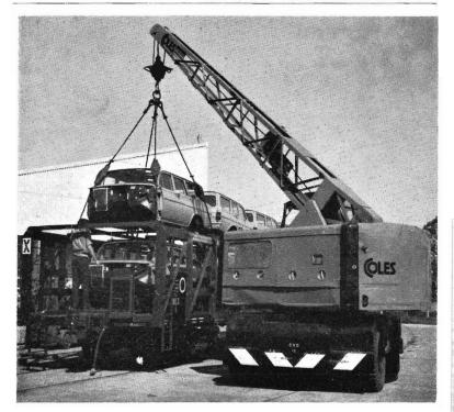
At General Motors-Holden's siding, Dandenong, a station wagon body is loaded on to the first of the new type of wagon for motor car bodies (See story above).
